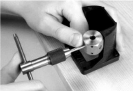
After using the Drill Bushing Kit to get the tap drill hole drilled straight in the motor mount, the Tap-N-Drill guide keeps the tap concentric with the hole.
