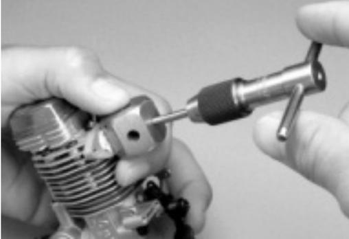
The Tap-N-Drill guide helps keeps tap perpendicular to the muffler mount surface while cleaning a gritty screw hole.
