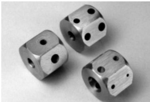
These tools keep the drill or tap perpendicular to the surface of the piece being tapped or drilled. The three-piece set handles common drills from 1/16" to 1/4" and all taps and tap drills from 0-80 through 1/4". The Guides are also available individually. We'll first show how to get wing bolts in straight.
